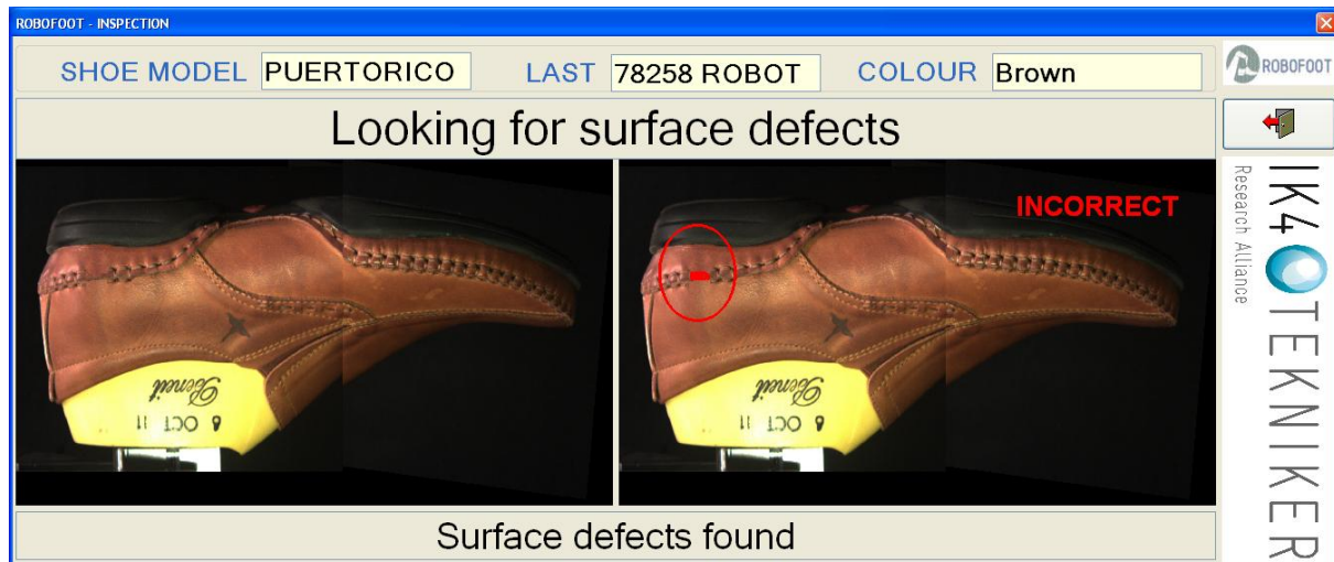
Fig. 7 Inspection result for surface defects detection
