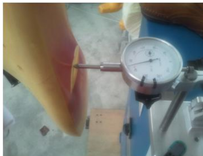
Fig. 20: Repeatability test using the dial gauge
