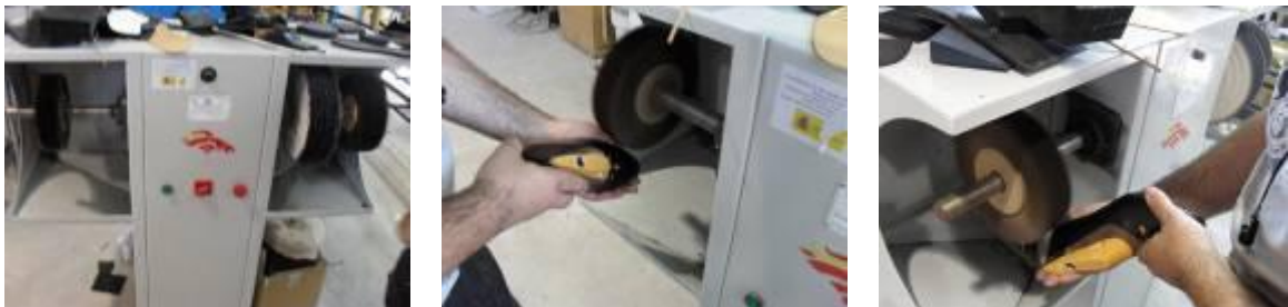
Fig. 15 Polishing process description
