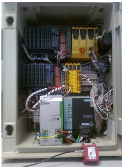
Fig. 29 Safe Rack with the two PLC and the Safe-PLC
