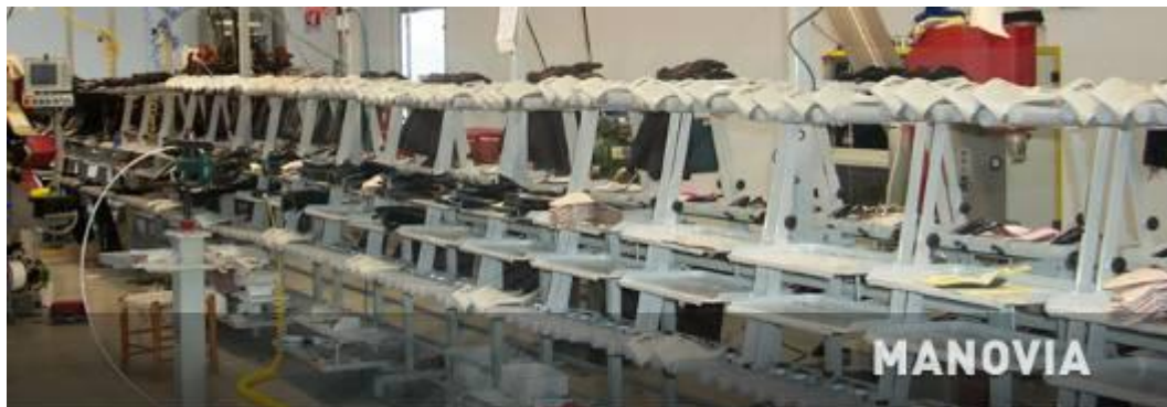
Fig. 10 Last over trolleys in a conveyor line
