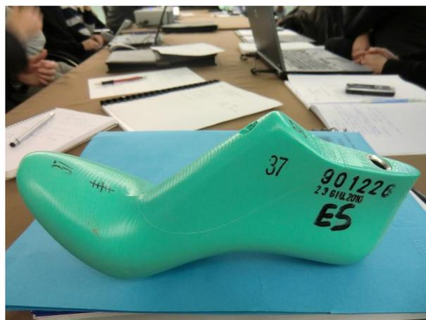
**Fig. 8 A last: the shoe is shaped on it**
