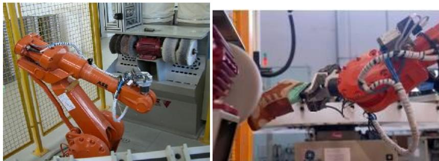
**Fig. 35 EUROShoE finishing cell**
