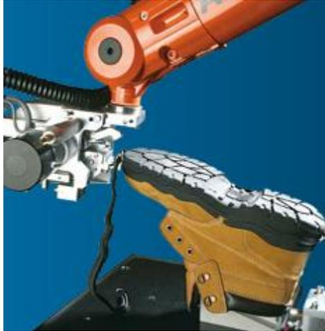
Fig. 44 – DESMA trimming robotised cell
