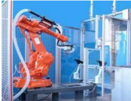
Fig. 40 – DESMA roughing and cementing robotised cell
