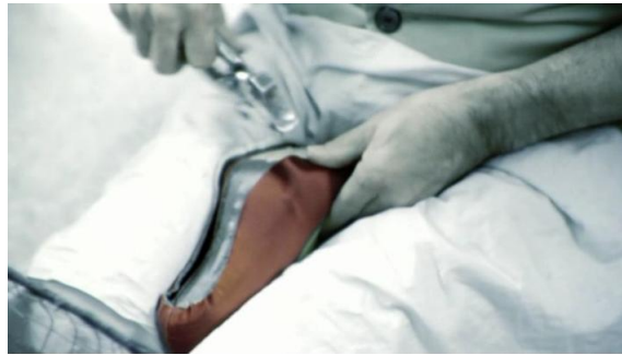
Fig. 32 To last the side leather
