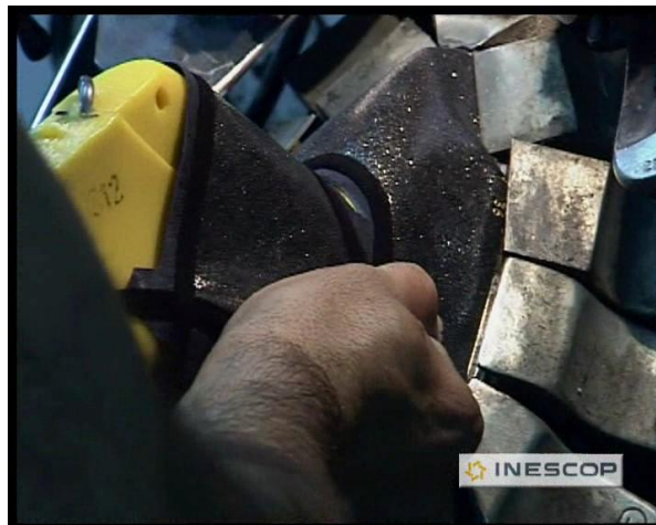
Fig. 31 Pulling over the last
