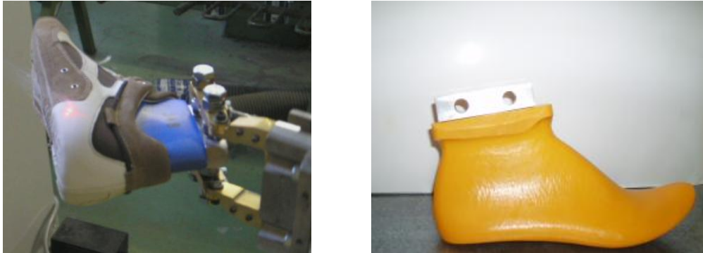
Fig. 39 Example of Gripping Method adding a fixture on top
